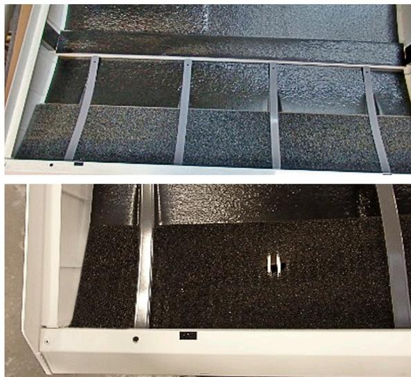
Note: For CDP/CDF 40 and 50 the filters must be cut according to this illustration.
